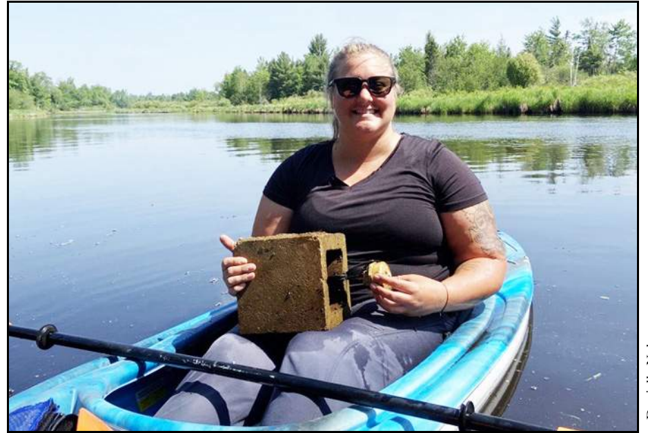
TEMP LOGGERS DEPLOYED ON THE WOLF RIVER WATERSHED Emma Balliet retrieves data from temperature loggers deployed in the Upper Wolf River Watershed.
